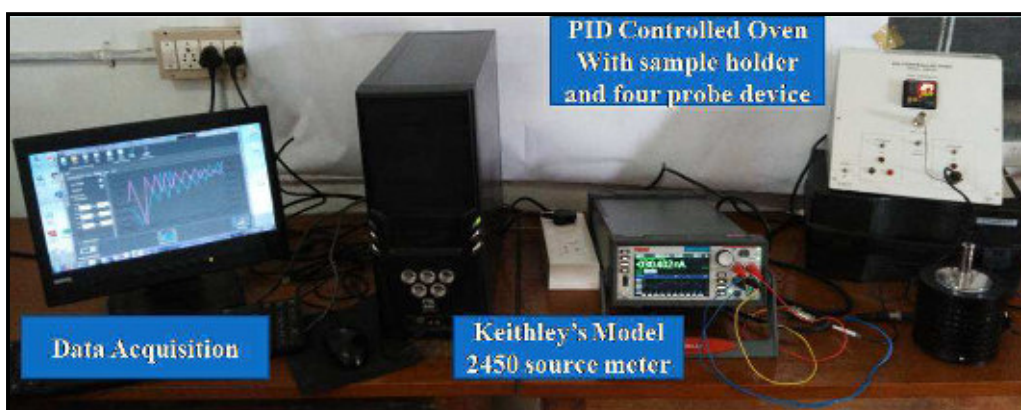
Fig. 2.7 Experimental set up for DC electrical studies
